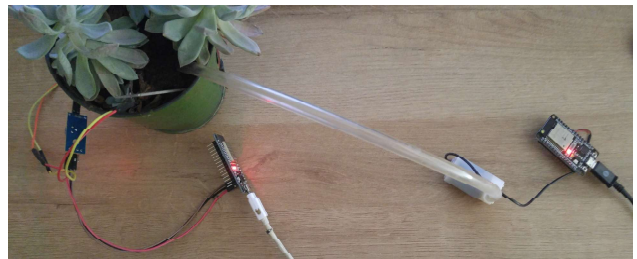
Figure 8: Setup for the smart irrigation system
